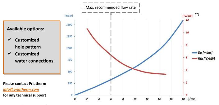
(\*) Rth :LCP surface to inlet water by homogeneous power loss distribution (Water + Ethylene Glycol 50%vol. @40°C)
